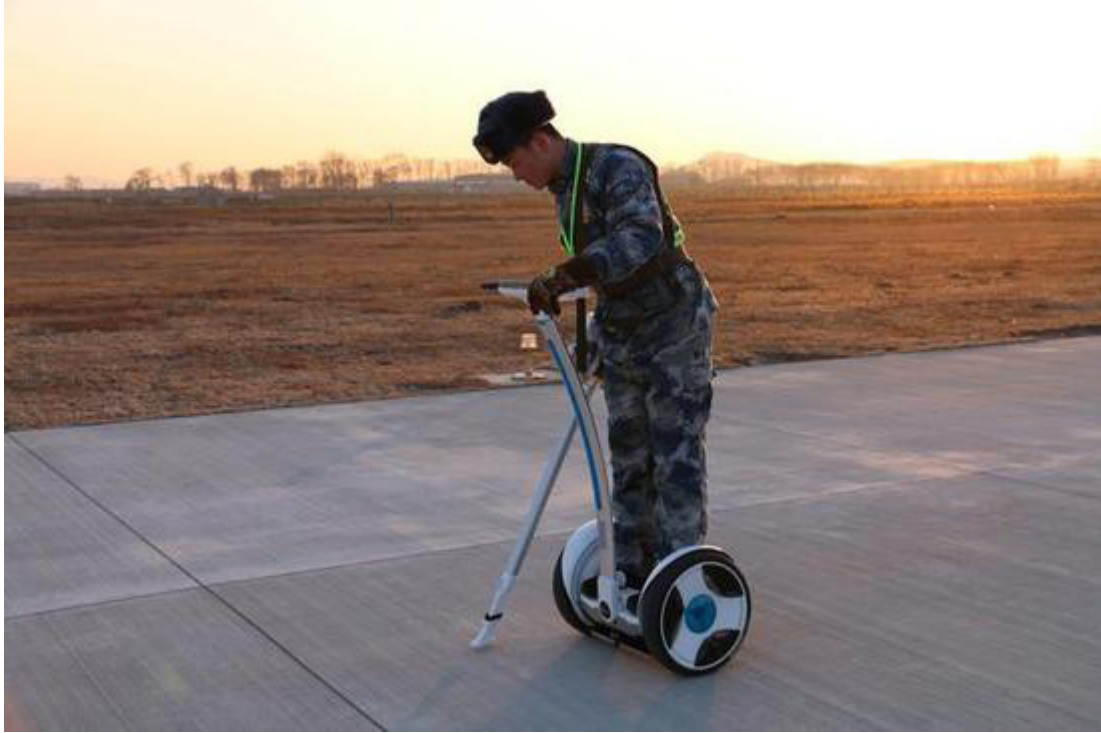
An airfield pavement individual rapid inspection device 44
